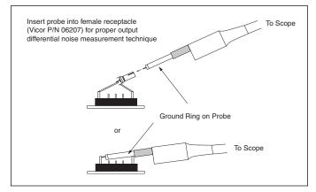
Figure 9–9 — Output ripple measurement technique
